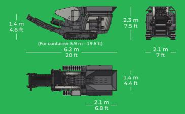
Recycling on site demolition and construction waste is a cost-efficient method of avoiding large landfill costs, onsite recycling and reducing demolition rubble to a useable product. The K-JC 604, a 600x400mm jaw crusher fitted with an integrated vibrating feeder, the material to be processed is moved in a fast, constant linear action into the jaw.
